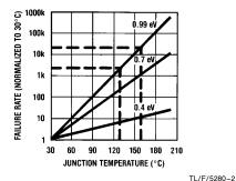
FIGURE 2. Failure Rate as a Function of Junction Temperature
